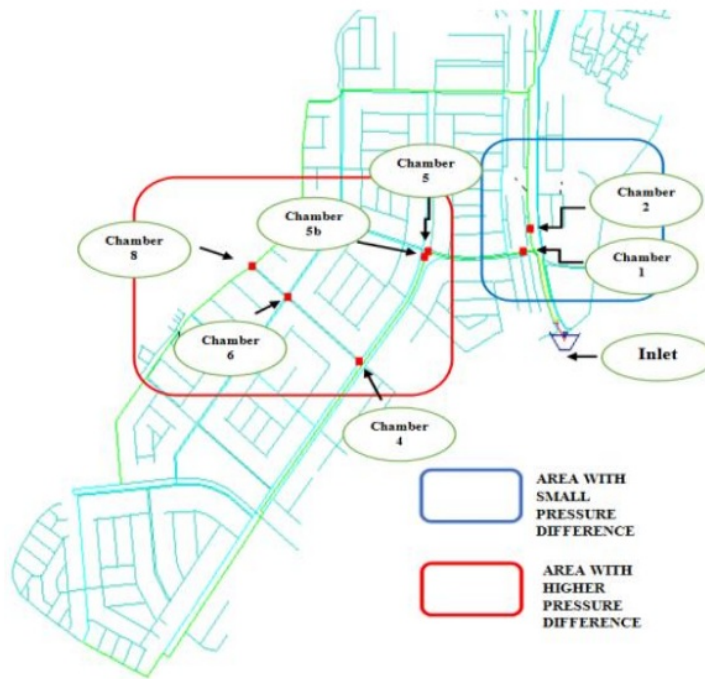
Figure 5. Placement of Pressure Monitoring Inside 7 chambers
