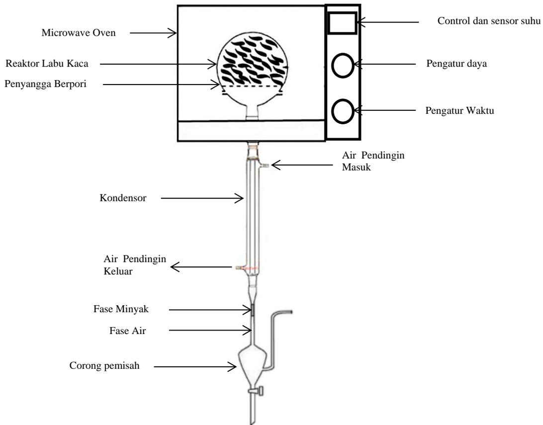
Gambar 1. Skema Alat Microwave Hydrodiffusion and Gravity (MHG)
