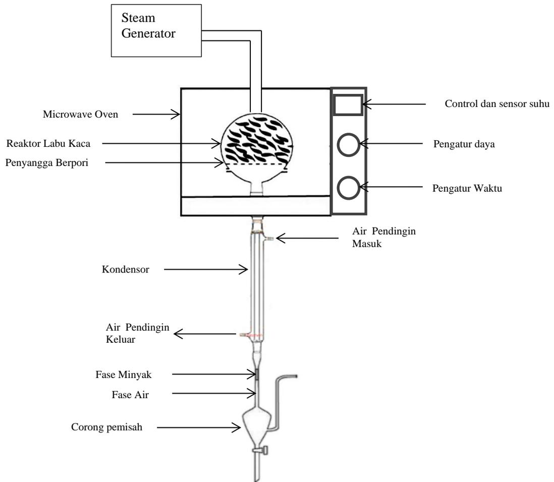
**Gambar 2. Skema Alat Microwave Steam Diffusion (MSDf)**
