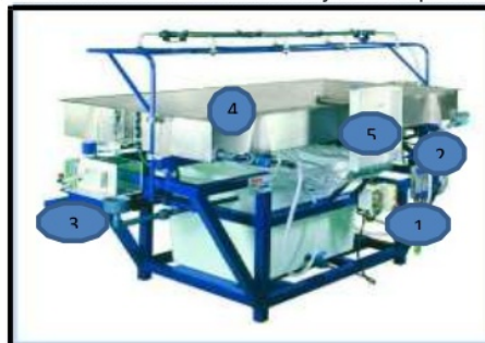
Figure 3. Rainfall Simulator S12-MKII Hydrology System, Armfield UK parts used in the machine are:
