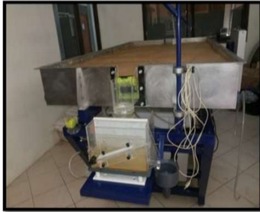
Figure 1. Rainfall Simulator of Hydrology System SK-III Armfield
