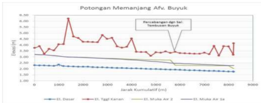
Figure 2. The influence of the tides in the Afv. Buyuk on P38 or 3.8 km from BB Permisan)
