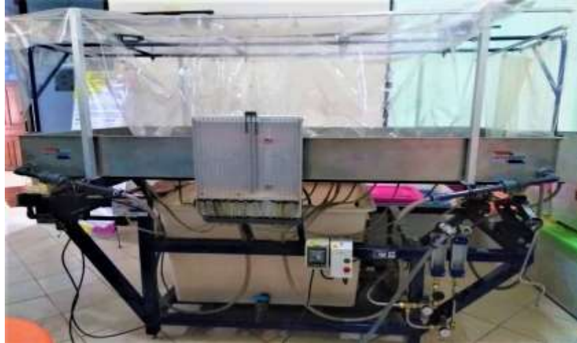
Fig. 1. Rainfall Simulator of Hydrology System SK-III Armfield Source: Own Documentation
